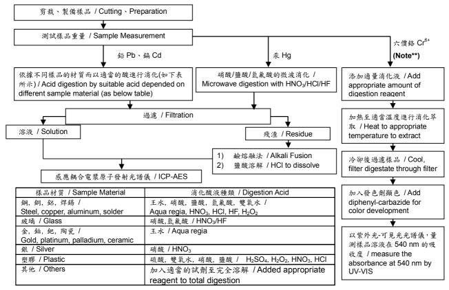
Note\*\*: (1) 針對非金屬材料加入鹼性消化液,加熱至 90~95℃萃取. / For non-metallic material, add alkaline digestion reagent and heat to 90~95°C
