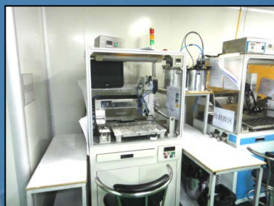
Equipment Name: Auto Black Glue Dispenser Brand: Science Origin : China Model: HDPG-3 Quantity: 2pcs
