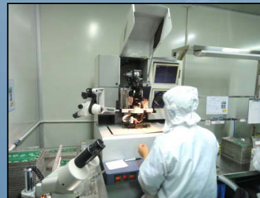
Equipment Name: COB Bonding Machine Brand: ASM Origin: Hong Kong Model: AB530 Quantity: 1pc
