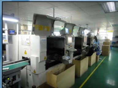
Equipment Name: SMT Machine Brand: JUKI Origin: Japan Model: KE-2050CM Quantity: 4pcs
