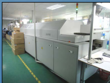
Equipment Name: Lead Free Reflow Machine Brand: SUNEAST Origin: Japan Model: IPC-8 Quantity: 2pcs
