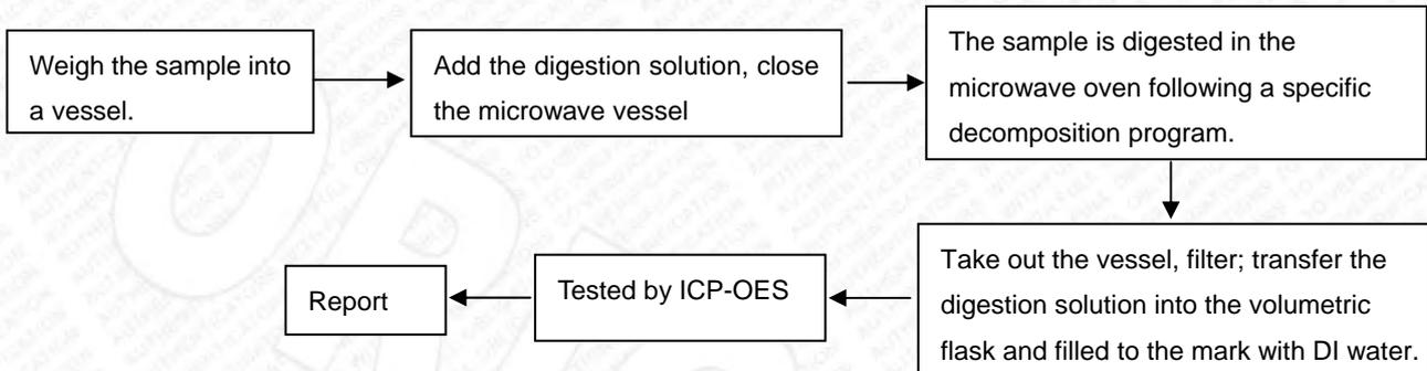
2. To Determine Lead, Cadmium Content (for metal):
