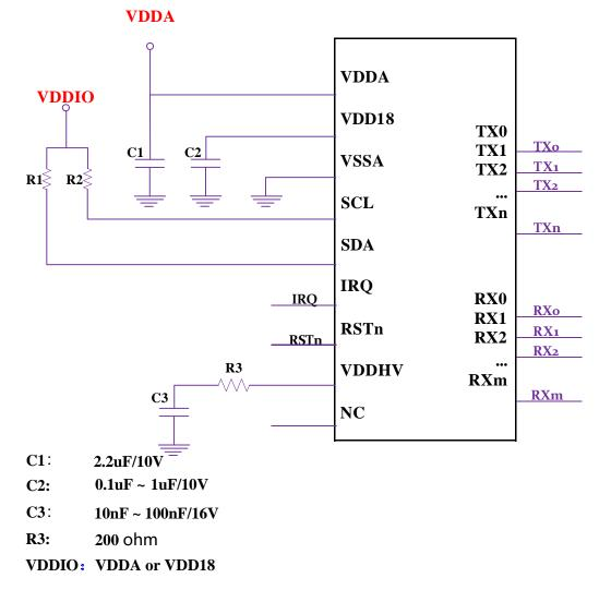
R1/R2 can be equipped with an optional I2C bus pull-up resistor. You can also configure the chip's internal 5K pull-up resistor to replace the Sensor ID. You can use the extra TX or RX to distinguish between two modes: floating or connected to GND.
