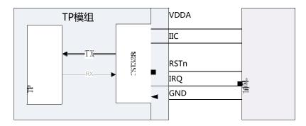
The above picture is the interface relationship between the host and CST328. The host and CST328 include IIC, IRQ, RSTn and VDDA signals. CST328
