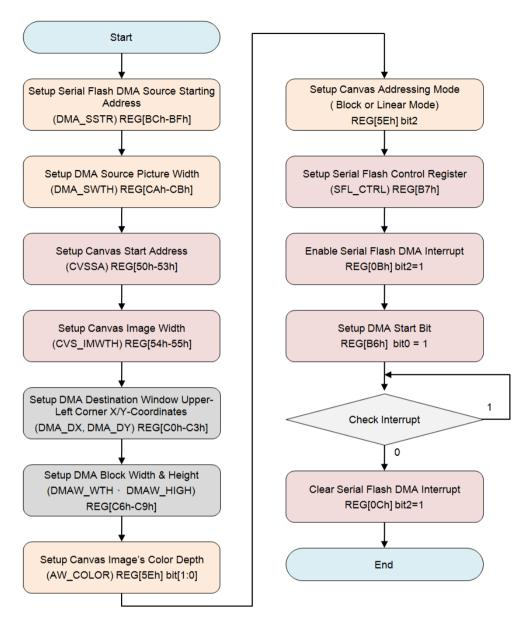
Figure 10-13: DMA Data Transfer Flowchart (Interrupt Mode)
