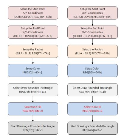
Figure 6-11: Flowchart of Drawing a Rounded-Rectangle
