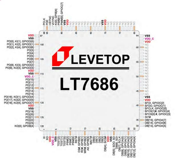
Figure A-4: LT7681/LT7683+/LT7686 Pin Assignment (LQFP-128Pin)
