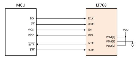
Figure 2-7: 4-Wire SPI Interface
