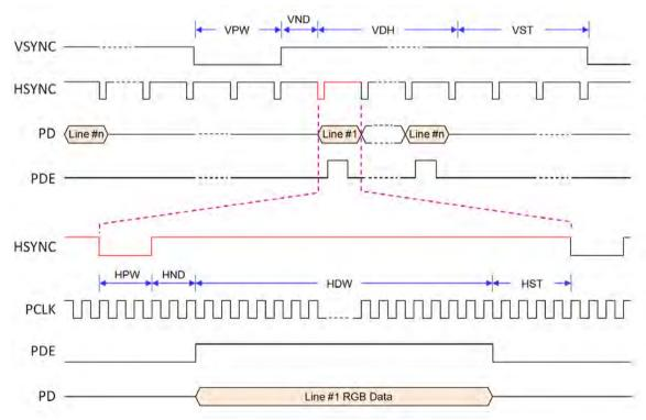
Figure 4-1: TFT-LCD Interface Timing
