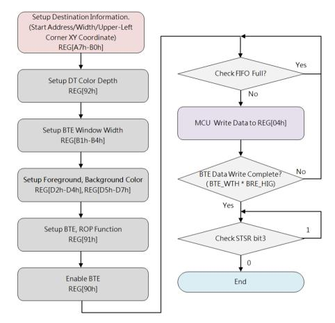
Figure 7-19: Flow Chart of MCU Write with Color Expansion
