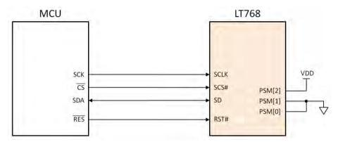
Figure 2-5: 3-Wire SPI Interface
