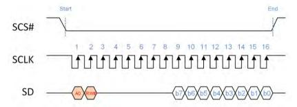
Figure 2-6: 3-Wire SPI Interface Timing
