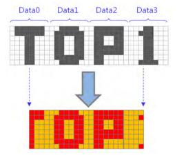
Figure 7-21: Example 2 of MCU Write with Color Expansion (ROP=3)
