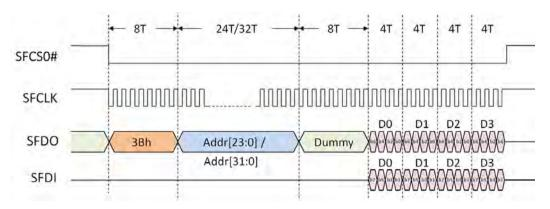
Figure 10-8: SPI Flash Read Command (Data and Address are Interleaved)
