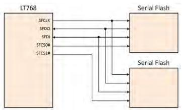
Figure 10-4: Application Circuit of Serial Flash/ROM
