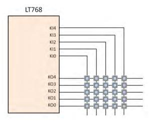
Figure 11-1: Application Circuit of Keypad-scan
