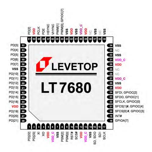
Figure A-5: LT7680A-R / LT7680B-R Pin Assignment (QFN-68Pin)
