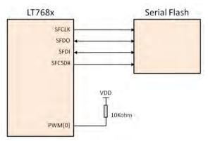
Figure 10-1: Enable the "Power-On Display" Function
