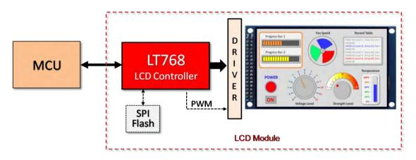
Figure A-3: LT768x Designed on TFT-LCD Module
