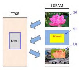
Figure 7-26: Example of Pixel Mode - 16bpp
