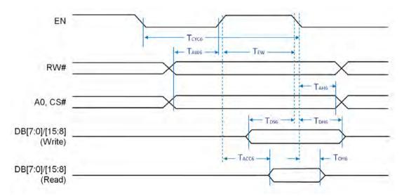
Figure 2-4: 6800 Parallel Mode Interface Timing
