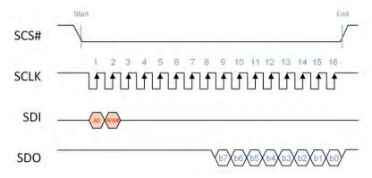
Figure 2-9: 4-Wire SPI Interface Read Timing
