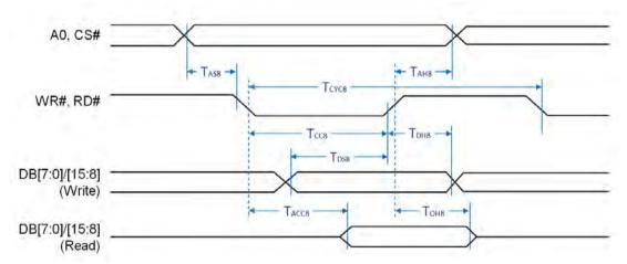
Figure 2-2: 8080 Parallel Mode Interface Timing
