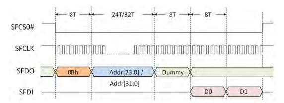
Figure 10-7: SPI Fast Read Command of SPI Flash
