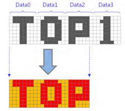
Figure 7-20: Example 1 of MCU Write with Color Expansion (ROP=7)
