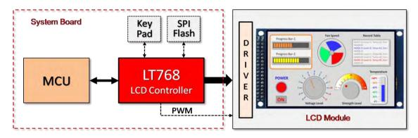
Figure A-2: LT768x Designed on System Board
