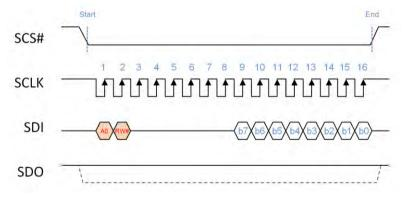
Figure 2-8: 4-Wire SPI Interface Write Timing
