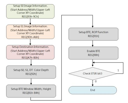
Figure 7-15: Flow Chart of Pattern Fill with ROP
