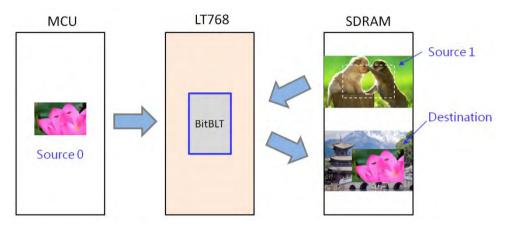
Figure 7-4: Example of MCU Write with ROP
