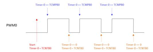
Figure 9-1: PWM0 Output Wave Form
