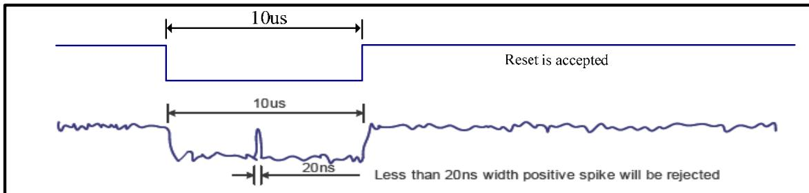
Note 5. It is necessary to wait 5msec after releasing RESX before sending commands. Also Sleep Out command cannot be sent for 120 msec.
