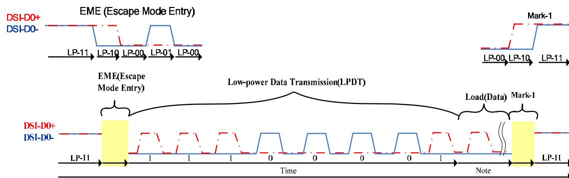
Note: Load(Data) is presenting that the first bit is logical "1" in this example.
