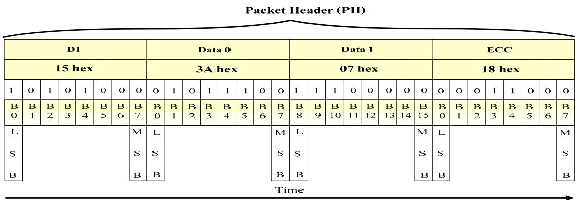
Figure: Packet head on short packet
