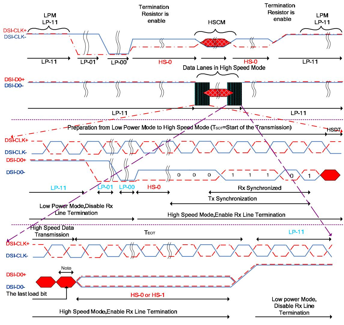
Figure: High speed clock burst
