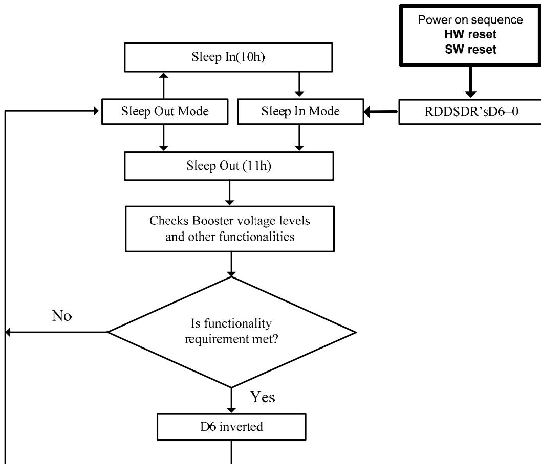
Note: There is needed 120msec after Sleep Out -command, when there is changing from Sleep In -mode to Sleep Out -mode, before there is possible to check if functionality requirements are met and a value of RDDSDR's D6 is valid. Otherwise, there is 5msec delay for D6's value, when Sleep Out -command is sent in Sleep Out -mode.
