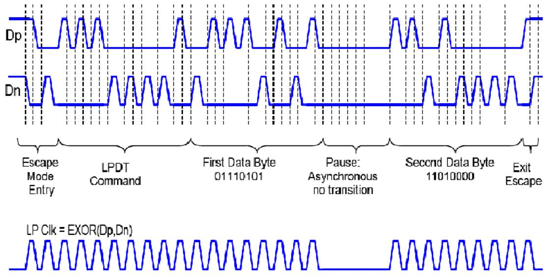
Figure: Two Data Byte Low-Power Data Transmission Example
