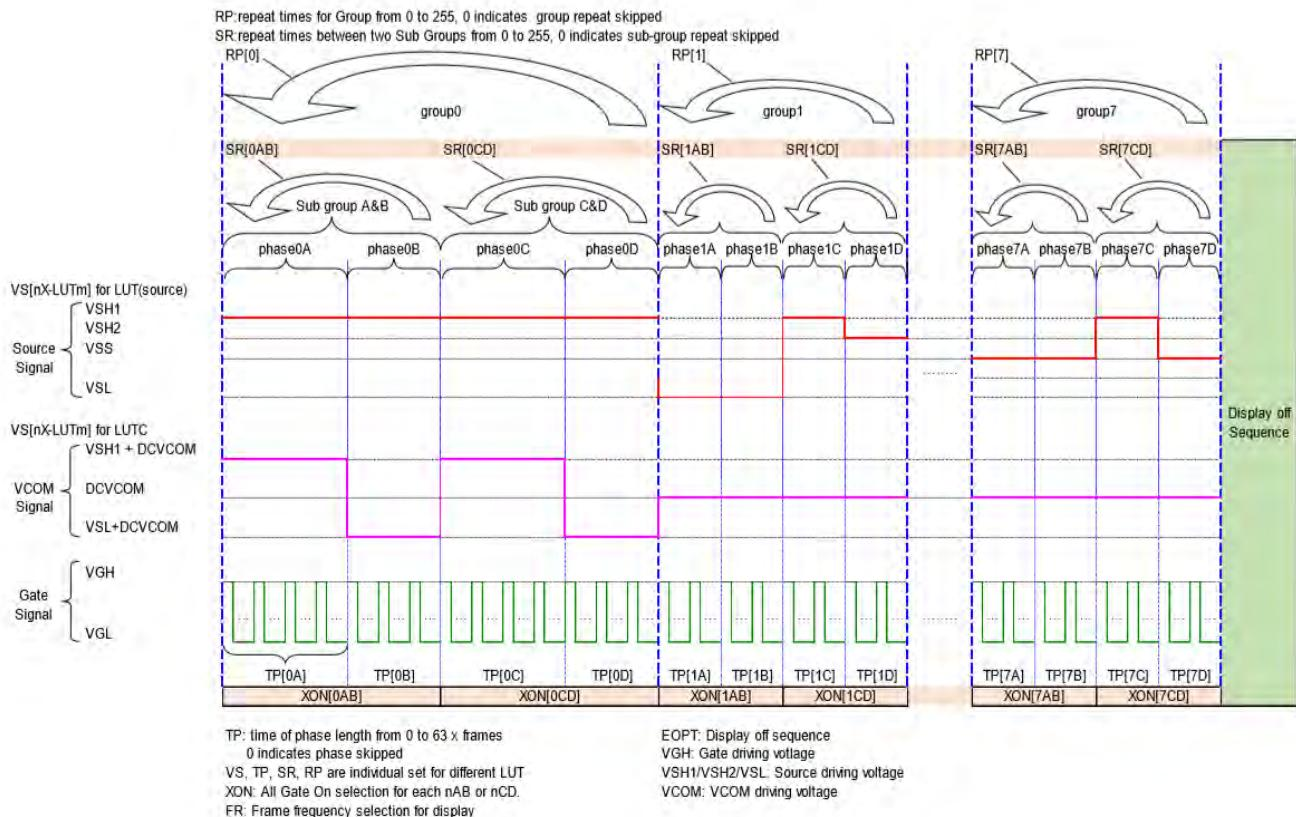
Figure 6-5 : Programmable driving waveform illustration
