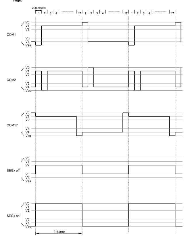
1/8 Duty(ST7066U normal mode); Assume the oscillation frequency is 540KHZ, 1 clock cycle time = 1.85us, 1/8 duty; 1/4 bias, 1 frame = 1.85us x 400 x 8 = 5.92ms=168.9Hz(SHLC and SHLS connect to
