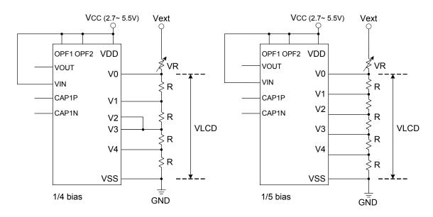
When built-in bias resistors(9.6K Ω) are used
