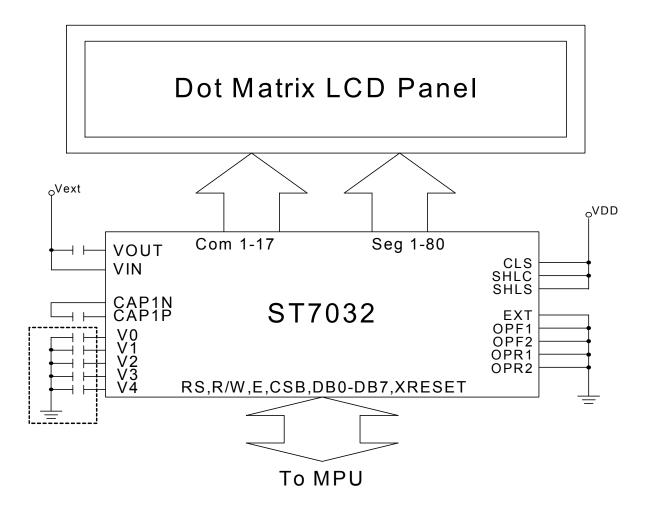
When the heavy load is applied, the dotted line part could be added.
