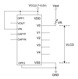
When built-in bias resistors(3.3KΩ) are used (OPF1=0,OPF2=1)
