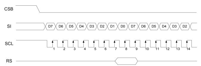
Note:The falling edge must cause on CSB before the serial clock ( SCL ) active.
