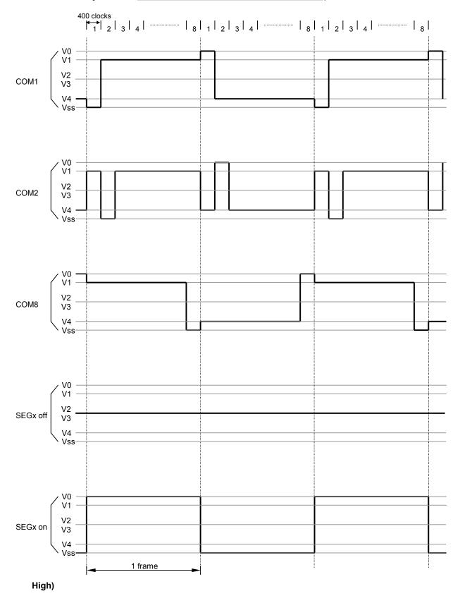
● 1/9 Duty(Extension mode); Assume the oscillation frequency is 540KHZ, 1 clock cycle time = 1.85us, 1/9 duty; 1/4 bias,1 frame = 1.85us x 400 x 9 = 6.66ms=150Hz(SHLC and SHLS connect to
