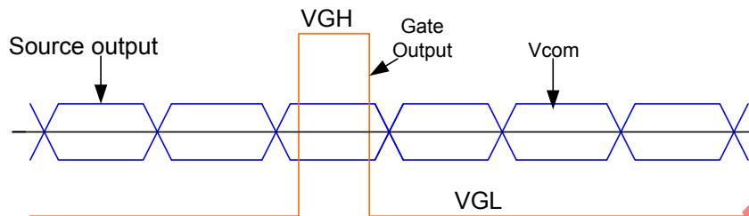
Figure 40 Voltage Output to TFT LCD Panel
