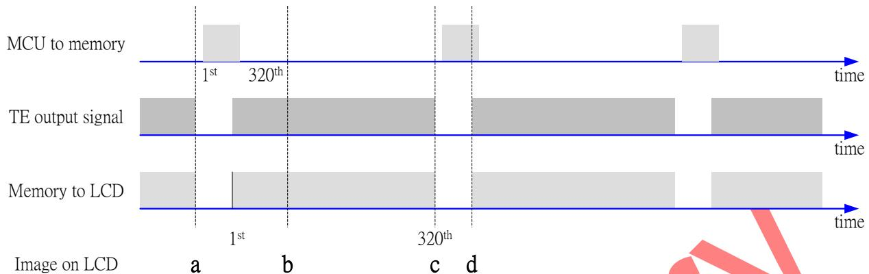
Data write to Frame Memory is now synchronized to the Panel Scan. It should be written during the vertical sync pulse of the Tearing Effect Output Line. This ensures that data is always written ahead of the panel scan and each Panel Frame refresh has a complete new image:
