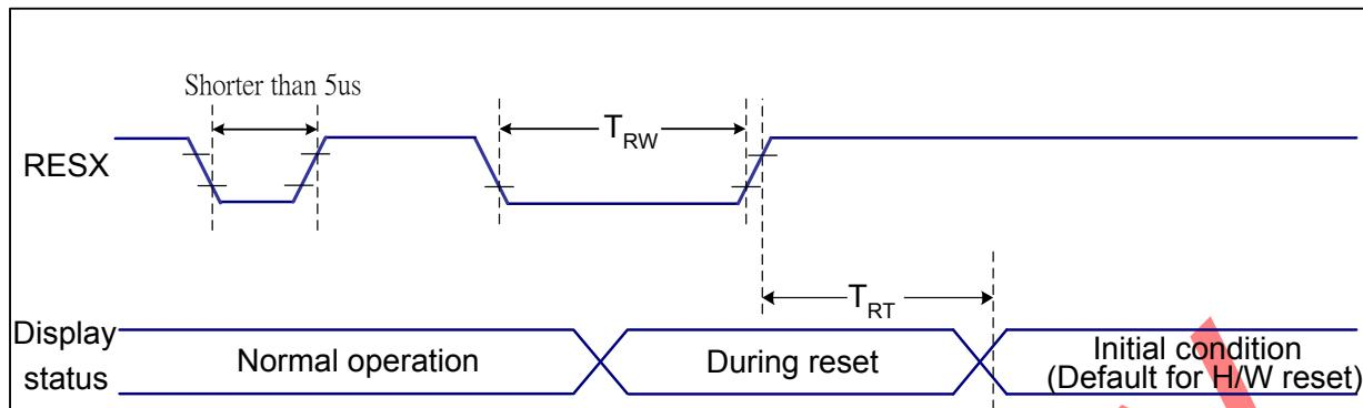
Figure 7 Reset Timing
