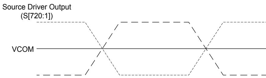
Figure 36 Relationship between Source Output and VCOM
