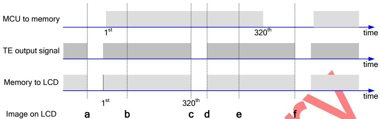
The MPU to Frame Memory write begins just after Panel Read has commenced i.e. after one horizontal sync pulse of the Tearing Effect Output Line. This allows time for the image to download behind the Panel Read pointer and finishing download during the subsequent Frame before the Read Pointer "catches" the MPU to Frame memory write position.
