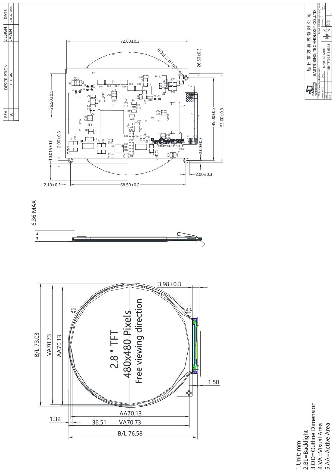
3.2 ER-TFT028-2-6318 with FFC Connection and with Capacitive Touch Panel Outline Drawing
