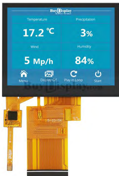
ER-TFT035-4 with Resistive Touch Panel →
