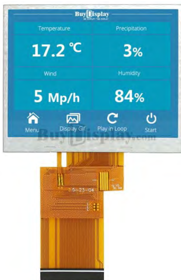
ER-TFT035-4 with Resistive Touch Panel →
