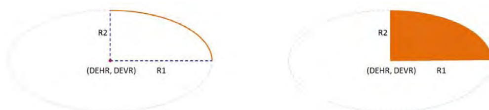
Figure 6-3: Drawing Curve and one-fourth Ellipse
