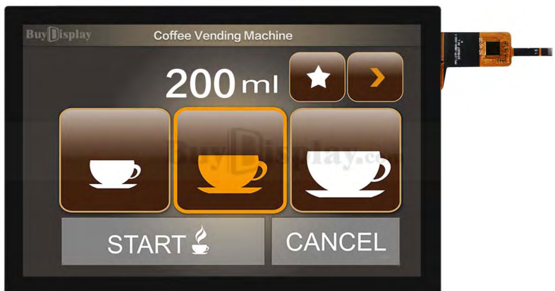
ER-TFT080-3 with Capacitive Touch Panel ↓
