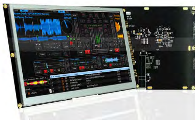
ER-TFTM080-1 with Resistive Touch Panel →
