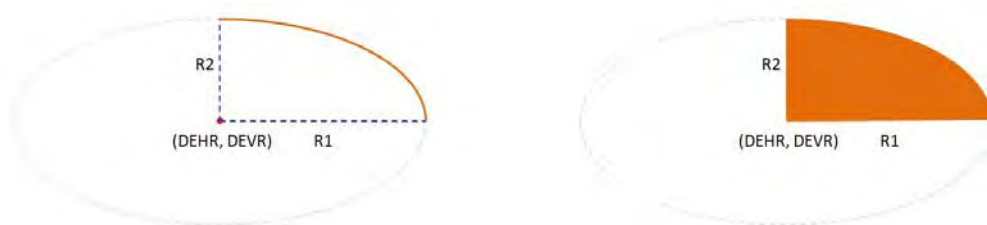
Figure 6-3: Drawing Curve and one-fourth Ellipse
